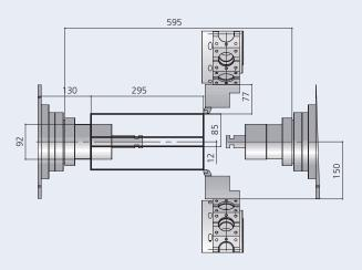
3 Simultaneous machining of T1 and T2 on M1
