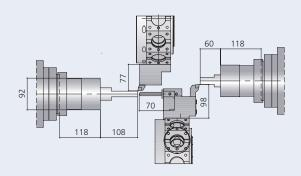
9 Simultaneous machining of T1 on M1 and T2 on M1 and M2 using three tools in "follow up" machining with Z2/Z3 thanks to the "Superimposition" function
