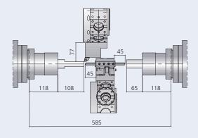
Simultaneous machining of T1 on M1 and T2 on M1 and M2 using three tools in "follow up" machining between Z2/Z3 thanks to the "Superimposition" function
