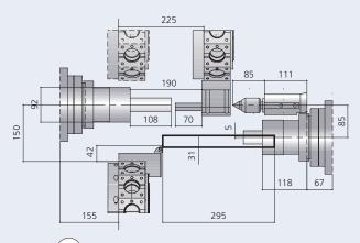
6 Simultaneous machining of T1 on M1 and T2 on M2 using tailstock
