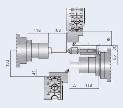
Simultaneous machining of T1 on M1 and T2 on M2 using tailstock to hold the component
