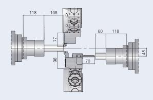
Simultaneous machining of T1 on M1 and T2 on M2 using three tools in "follow up" machining with Z2/Z3 thanks to the "Superimposition" function
