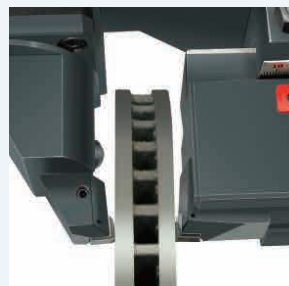
Simultaneous dual-face turning of disk brake
