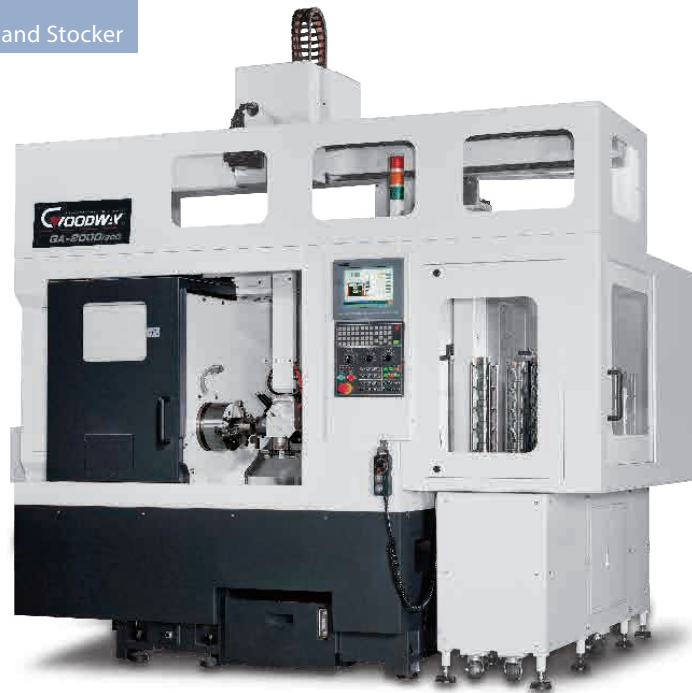
( Gantry Loading with GOODWAY GA-2000/300 series )
