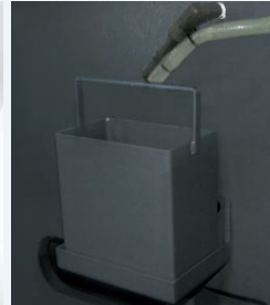
Built-in lub. oil collection system
